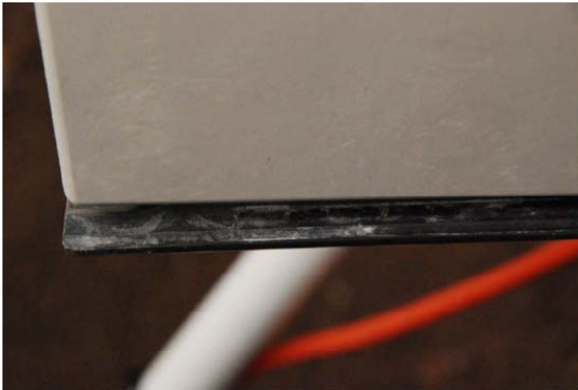
Figure 6: GRIMM sampler - soiled by dust
