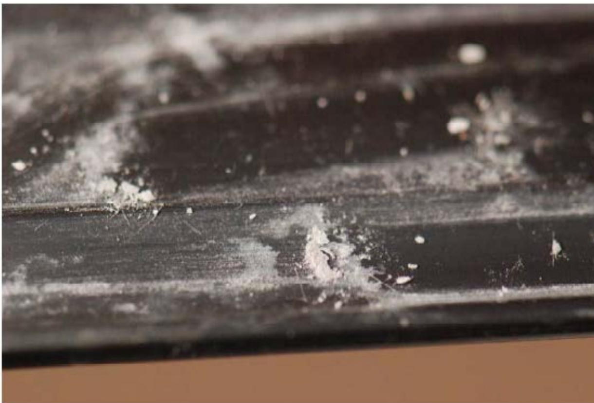
Figure 7: GRIMM sampler - close-up of soiling
